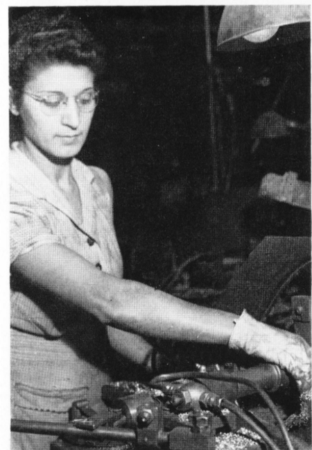
Susan Coleman, of Chucking, places a ring on the chuck. Reversible cotton gloves, which last only a day, protect her hands from the ragged edge of the forging, and from heat.
