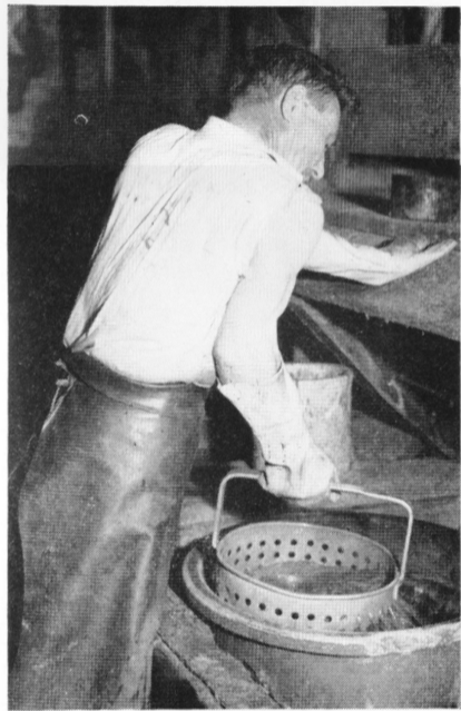
High grade rubber gloves are best suited for work in the Dip and the Lacquer Rooms. Guiseppe Ortale, Dip Room, is wearing a pair of heavy rubber mittens against acids hazards.
