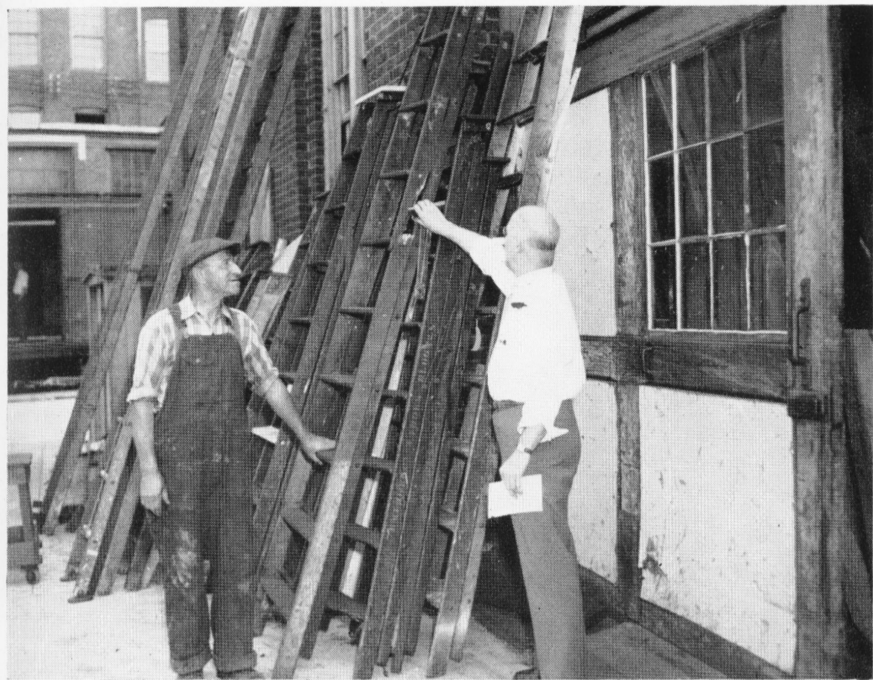
Oscar Hubbell, Carpenter Shop, and Walter J. Racicot, Health and Safety, are examining some broken ladders by the Carpenter Shop, awaiting repairs. Some are "suffering" split rails, broken rungs, broken shoes, bracers and spreaders. Check ladders before using.
